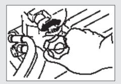
While pump is in operation care should be taken to ensure that it is not tilted more than 30° off the horizontal in any direction. The pressure relief valve must not be opened while the cutter is in operation.
