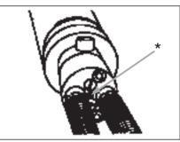
Immediately switch the relay valve of the hydraulic power unit into neutral position and reconnect the couplings correctly.
