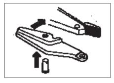
In order to tighten the chain push the catch any one time – tighten the chain as strong as possible – close the blades (arms).
