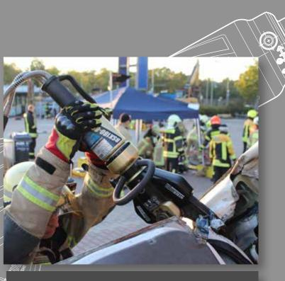
Lower tension on blades due to the optimal cutting angle and edges plus overlapping design
