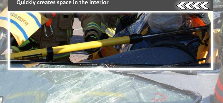
Perfect for enlarging collapsed and deformed interior vehicle space and aid working within the vehicle
