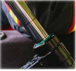
Laser-etching on the piston rod - always see the remaining length!
