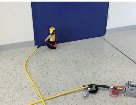
The third option is to use the door opening cylinder underneath the door to lift it out of its hinges, or to weaken the lock and any bolts that may be present before breaking them open.
