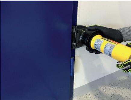
Breaking open a the door hinge is the second option. This works particularly well if the door opens outwards and the hinges are therefore directly visible.
