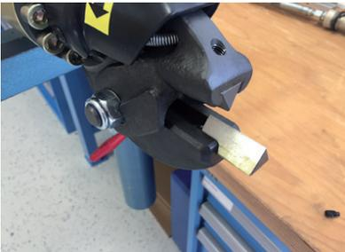
The rotated or replaced blade can then be pushed back in. Ensure that the closed side of the two slots points forwards so that they can be gripped again when being replaced again.
